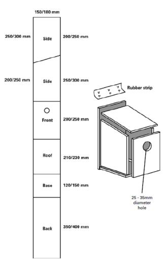
2. Nail the sides to the back with three nails on each side
